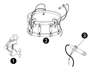
**WARNING:** Do NOT tighten the thumbscrew on the plastic section of the connector as this could cause damage.
