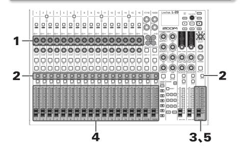
**1.** Use to adjust the input signals while inputting sound from instruments and mics.
