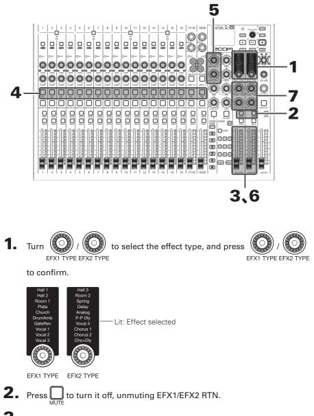
Set the EFX1/EFX2 RTN fader to 0.
