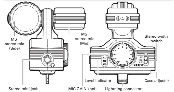
**M-S stereo mic:** This is a mid-side stereo microphone. Turn to change its orientation. (See "Changing the mic orientation.")
