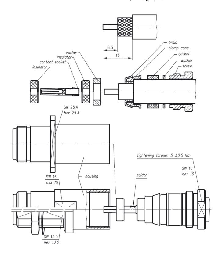
48-807 TG N CONNECTOR Female cable, solder, groups C/T Cable prep and assembly diagram
