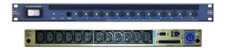
Power manager mains distribution unit, 12 way, 16 x GPIs, ethernet output monitoring and alarms – email and SNMP, individually controlled latching relays, sequential & delay power up with current sense network monitoring.
