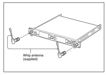
**3** Use commercially available BNC cables (50  $\Omega$ , 60 cm or longer) to connect the antenna mounts with BNC connectors to the ANTENNA a/b IN connectors on the rear panel of the unit.
