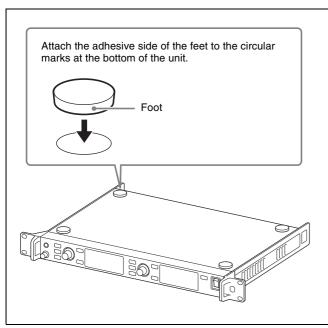
To install the unit in the rack, be sure to remove the attached feet.
