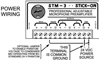
NOTE: THE STM-3 WILL OPERATE (WITH REDUCED HEADROOM) ON SUPPLY VOLTAGES FROM 9 TO 23 VDC.
