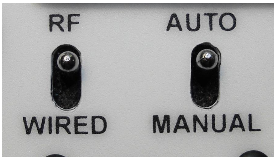
Photo showing proper setting of mode switches for use with RF remote control
