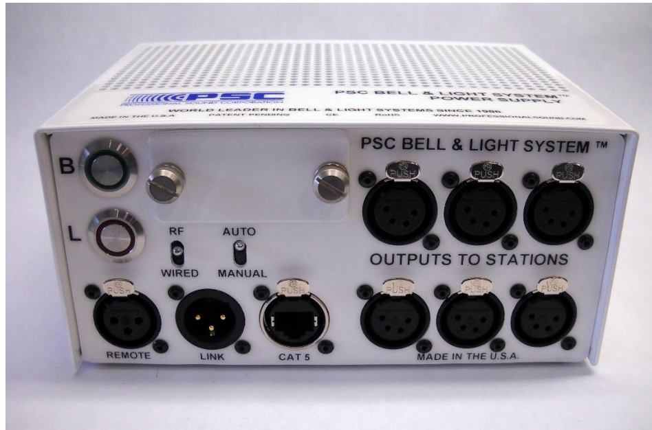
Photo showing blank cover plate in place before installing RF receiver Module. You must remove this access cover plate by unthreading the two thumb screws.
