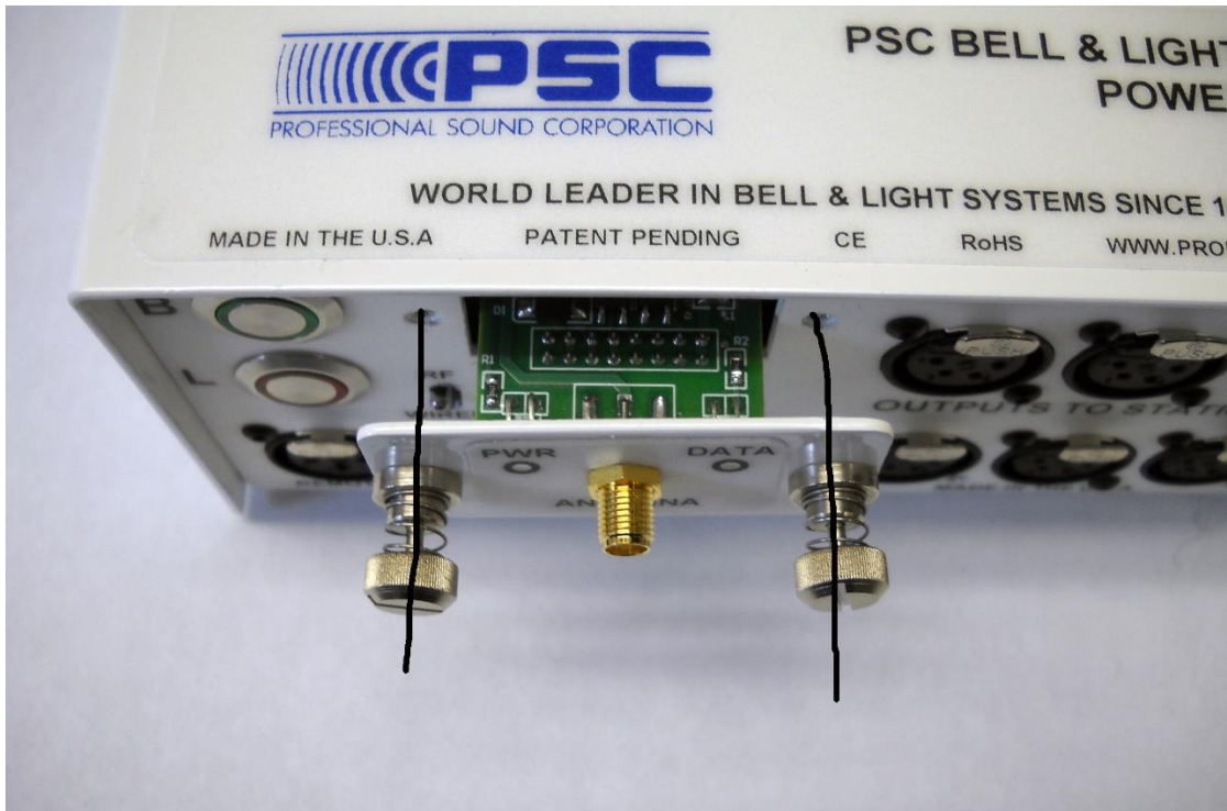
Photo showing how thumb screws must be aligned with threaded holes on Power Supply
