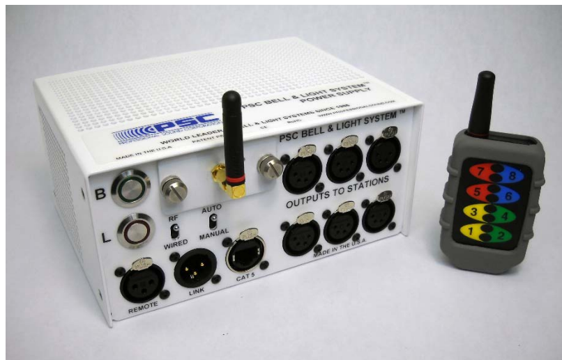
Option RF Receiver Module Installed in the Power Supply and Hand Held RF Remote Control
