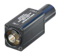
Female BNC 75  $\Omega$  input - male XLR cable type connector 110  $\Omega$  output. For matching balanced 110 ohm digital audio circuits to unbalanced 75 ohm video circuits.
