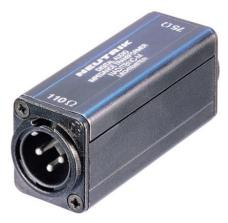
Female BNC 75  $\Omega$  input - male XLR chassis connector 110  $\Omega$  output. For matching balanced 110 ohm digital audio circuits to unbalanced 75 ohm video circuits.
