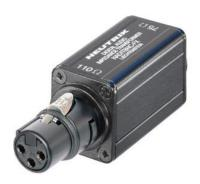
Female XLR cable type connector 110  $\Omega$  input - female BNC 75  $\Omega$  output. For matching balanced 110 ohm digital audio circuits to unbalanced 75 ohm video circuits.
