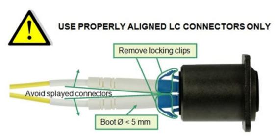
Avoid splayed connectors by using LCs without anti-snag collars and a boot diameter < 5 mm (available from suppliers as e.g. Corning).
