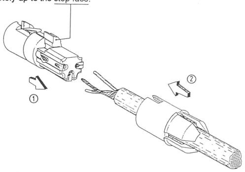
Note: There are two possible positions the chuck can be assembled. You can choose whether or not the housing will be grounded (connected to contact '1') by rotating the chuck 90°.
