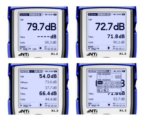
The Extended Acoustic Pack, when installed on your XL2, supports the daily tasks of acoustic consultants. It offers additional features for sound level logging and acoustic measurements, such as recording linear wav-files, percentile statistics, sound exposure level, 100 ms logging, event monitoring, reverberation time in 1/3 octave resolution, Zoom-FFT with 0.4 Hz resolution and many more.
