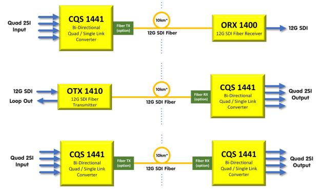
A fiber Transceiver option is also available. This includes both a Transmitter and Receiver in a single SFP package. The receive and transmit functions cannot be used simultaneously, but this option is useful if the CQS 1441 configuration is frequently changed where fiber transmission is sometimes needed and on other occasions fiber reception.
