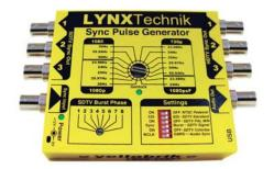
Every non-linear edit system working in conjunction with a VTR requires a stable reference signal in order to lock everything together to ensure timecode accurate editing. The SPG 1707 provides this much needed stability.
