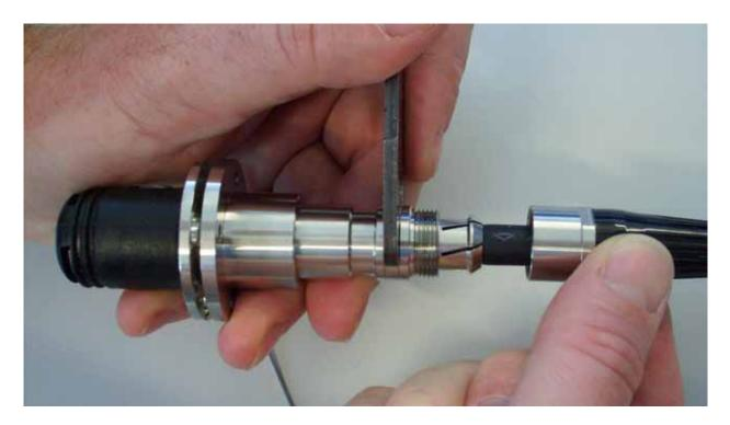
4. Using the spanners release and un-screw the extended shell.
