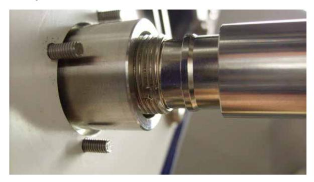
9. Using the spanner tighten up the rear extended housing.
