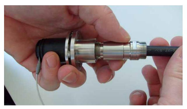
6. Remove the inner assembly taking care not to disturb the centre pieces.
