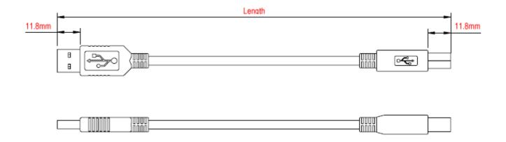
38-752 USB CABLE 2.0, Type A male - Type B male, LFH, 2 metre 38-753 USB CABLE 2.0, Type A male - Type B male, LFH, 3 metre
