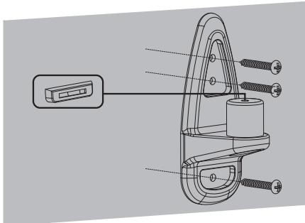
Use a pencil to mark the place for mounting. Make sure the wall structure can support the weight of monitor along with the mount. Avoid dead center for mounting holes.
