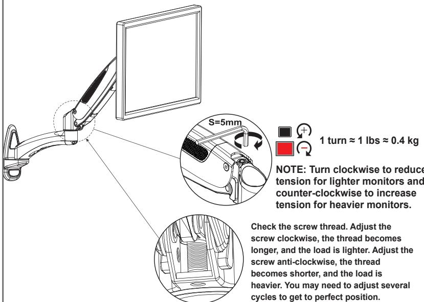
Use a hex wrench to adjust the height tension of the gas spring arm, to keep different weight of monitors still at any position.
