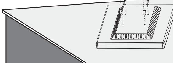
Recessed surface installation: Put 4 spacers between faceplate and monitor. Install 4 screws through faceplate, spacers to monitor via mounting holes.
