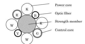
Attached drawing Cross section drawing of 2SM-16-37.5
