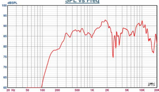
Sound pressure levels at 1W/1m closed 90° SPL vs Freq
