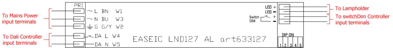
EASEIC LND127 AL art633127 LED driver with mains power input and Dali control input on left, LED lamp output, switchDim control and Dip Switches on the right as illustrated. *Note, there are other versions of this driver where the mains and control inputs are not arranged as illustrated. If such a driver is installed to the Script Light the following reset will not work and should not be undertaken.*
