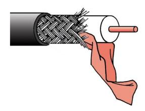
75 ohm coaxial cable designed for CCTV, CATV, satellite TV and RF signal distribution. CT167 cable has a water and UV resistant PE (polyethylene) jacket suitable for external and underground duct applications.
