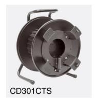
Robust cable-drum, steel drum with steel tube frame. Friction drum-brake incorporated into the frame to prevent movement in transit. 'Cable tail' type drum with solid steel flange open hub plus four brackets on the flange face to enable the cable tail to be brought out from the hub of the drum at a gentle angle (important for coaxial and essential for fibre cables) and coiled and secured around the brackets.. Fixed handle. Black finish.
