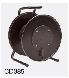
Black steel cable drum, with steel tube frame. Friction drum-brake incorporated into the frame to prevent movement in transit. Removable plastic blanking-plate over the hub, which can be punched to accept connectors as required, or removed for access to the inner tail of the cable. Folding winding-handle on the drum flange.
