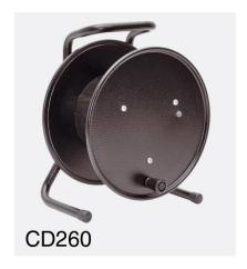
Robust cable-drum, steel drum with steel tube frame. Friction drum-brake incorporated into the frame to prevent movement in transit. 'Plain' type solid steel flange. Fixed handle. Black finish.
