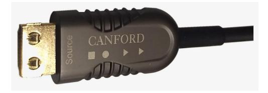
Active, optical, HDMI 2.0 cables intended for deployable applications where longer cable lengths than those obtainable with standard copper HDMI cables are required, (typically 10 - 15m max). They are also useful where the cable needs to pass through environments with high electrical interference. They offer a considerably more elegant and cost-effective solution for long cable runs than Cat5E cable with converter box systems.
