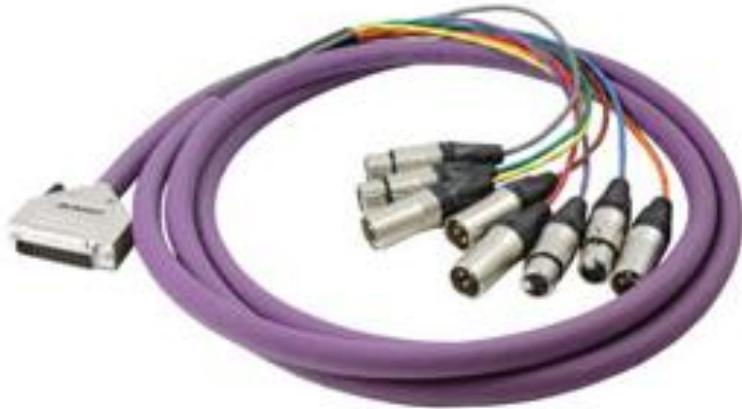
Suitable for AES digital audio I/O this cable assembly is wired to the Tascam convention. Belden 7880A low-capacitance, individually screened, 110 Ohm eight-pair cable used. The D-sub 25-pin male connector has a metal-body and sensibly-sized thumb-screws.
