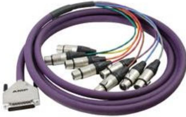
Suitable for Analogue audio input this cable assembly is wired to the Tascam DTRS convention. Belden 7880A low-capacitance, individually screened, 110 Ohm eight-pair cable used. The D-sub 25-pin male connector has a metal-body and sensibly-sized thumb-screws.
