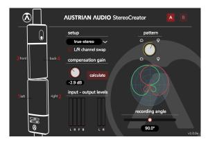
From the very beginning, musicians, composers and sound engineers have used the OC818 for stereo recordings. You can use just one OC818 in dual mode or attach a second microphone. You can then use the StereoCreator plug-in to choose between different stereo recording techniques such as X/Y, M/S or Blumlein.
