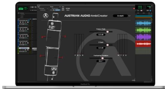
With our AmbiCreator plugin we go one step further—getting an ambisonic B-format signal out of two OC818 microphones, e.g. a “Live-Set”. As the OC818 microphones have a dual output, we can calculate any first-order pattern from those two outputs.
