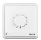
The Apart E-VOLST is a 4 ohms, low impedance stereo volume control that can handle up to 2 x 40 watts of power. It is very versatile thanks to the step-by-step attenuation in 6 steps.
